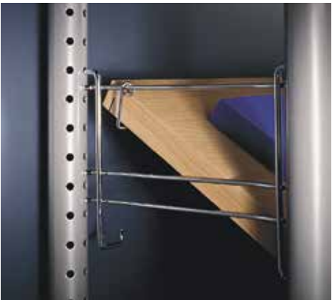
Slanting hook, Model SSTH For extractable shelves respectively metal or wooden shelves with projection, prevents the forward tilt of the shelf in the bay; two tilt securings required per shelf, black plastic.
