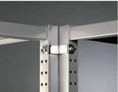
Corner connection angle, Model EVW For connecting the bearing frames of two shelving sections across the corner, for an even distance between the shelves. Two each are required per shelf connection. Nickel-plated metal, incl. fastening kit.
